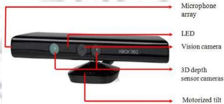
**Figure 1. Kinect Sensor.**
