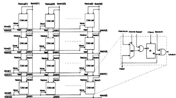
Fig .6. CAM based dictionary Architecture
