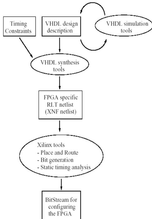
Fig.3. FPGA synthesis and implementation steps
