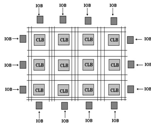
Fig.4. Basic Architecture of FPGA
