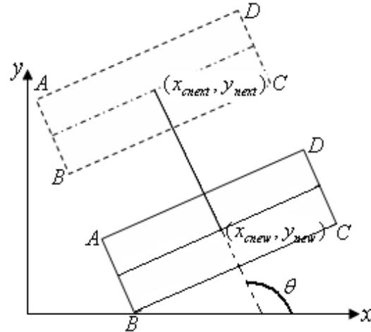
Fig. 2. Current (solid line) and next position (dashed line) of the box after translation.
