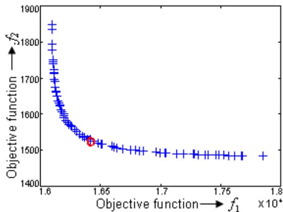
Fig. 5(b). Non-dominated solutions with NSGA-II for step 3.
