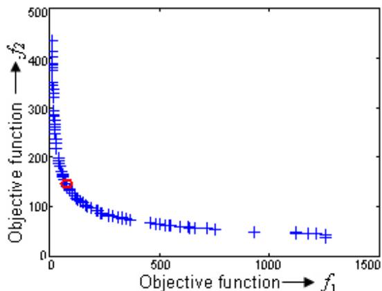
Fig. 5(c). Non-dominated solutions with NSGA-II for step 6.
