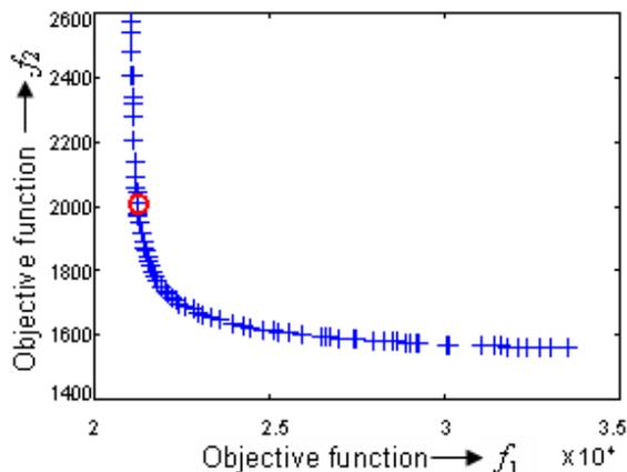
Fig. 5(a). Non-dominated solutions with NSGA-II for step 1.
