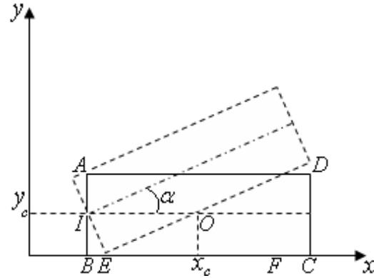
Fig. 1. Position of the box before (solid line) and after rotation (dashed line).
